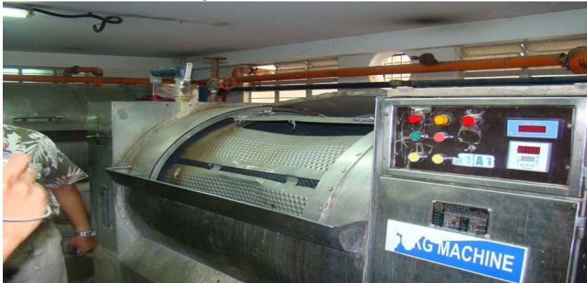
Figure No. 6: Washing machine showing circular 0.65 cm sized uniformly arranged, centrally perforated elevations over inner drum and on right side switch buttons without safety guard.
